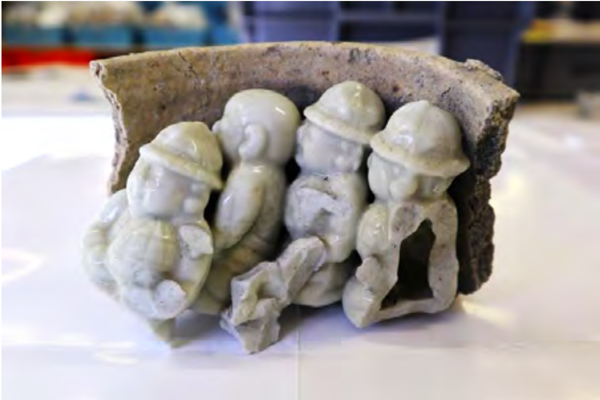
Figure 1. An example of figurine production in Seto from the early 1900s. Press-moulded pieces have been fused together in a saggar. (Photo: The author, 2019. Courtesy of the Seto City Archaeology Resource Centre)
