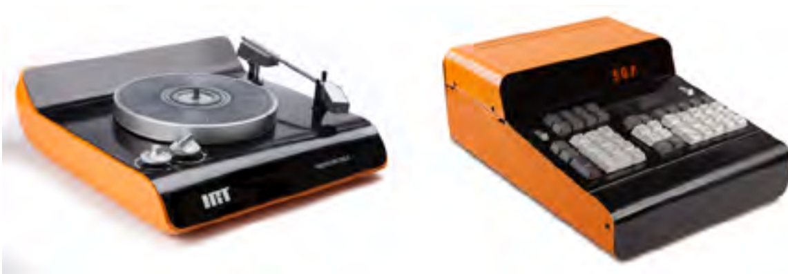
Figure 5: (left) Reconstruction of Portable Turntable. Fiberglass, latex, self-adhesive vinyl, original components of IRT Capissimo turntable. (right) Reconstruction of electronic calculator. Electronic Table Calculator. Steel, enamel, mechanical buttons, nixie tubes, acrylic, electronic components, Raspberry Pi, Phyton. Photo: Andrés Cortínez
